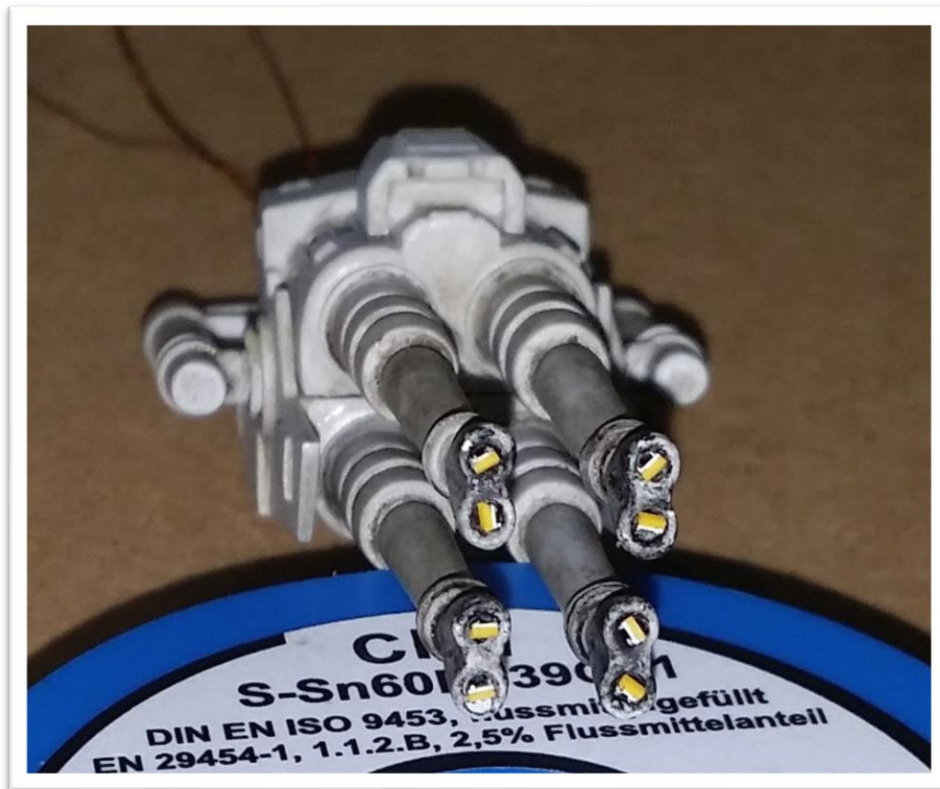
Figure 13 shapeways quadgun equipped with 0401 LEDs
