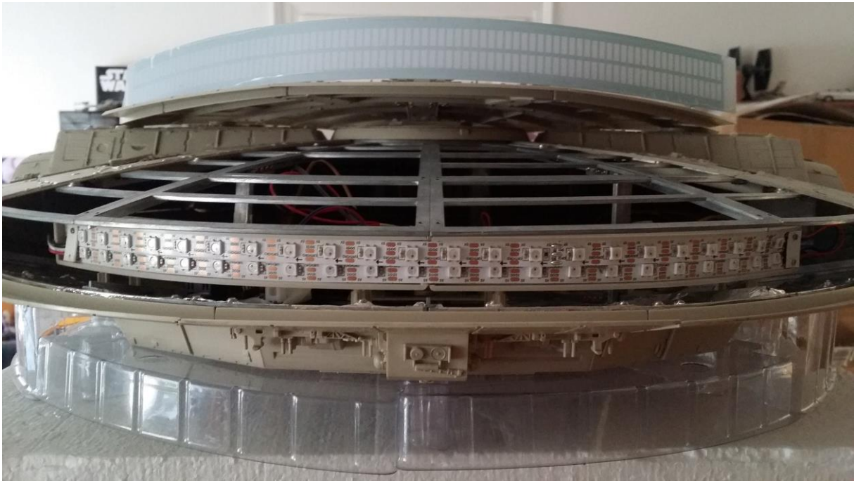
Figure 21 2x22 LED Neopixel strips
